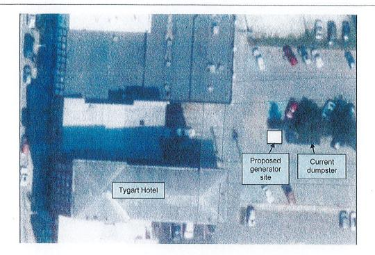
PROPOSED EMERGENCY GENERATOR LOCATION GENERATOR APPROX 8'-1"x3'-4" FENCED ENCLOSURE 20'x14'
