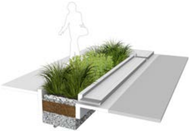
Vegetated buffers along sidewalks can filter stormwater from the roadway through a series of curb apertures.
