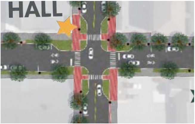
Intersection upgrades at 4th Street and Davis Avenue highlight paver sidewalk detailing and new striping.
