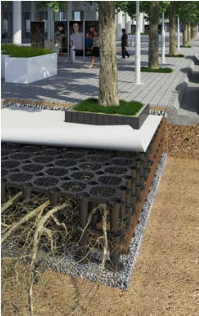
3D Visualization of a structural cell system used for street tree planting
