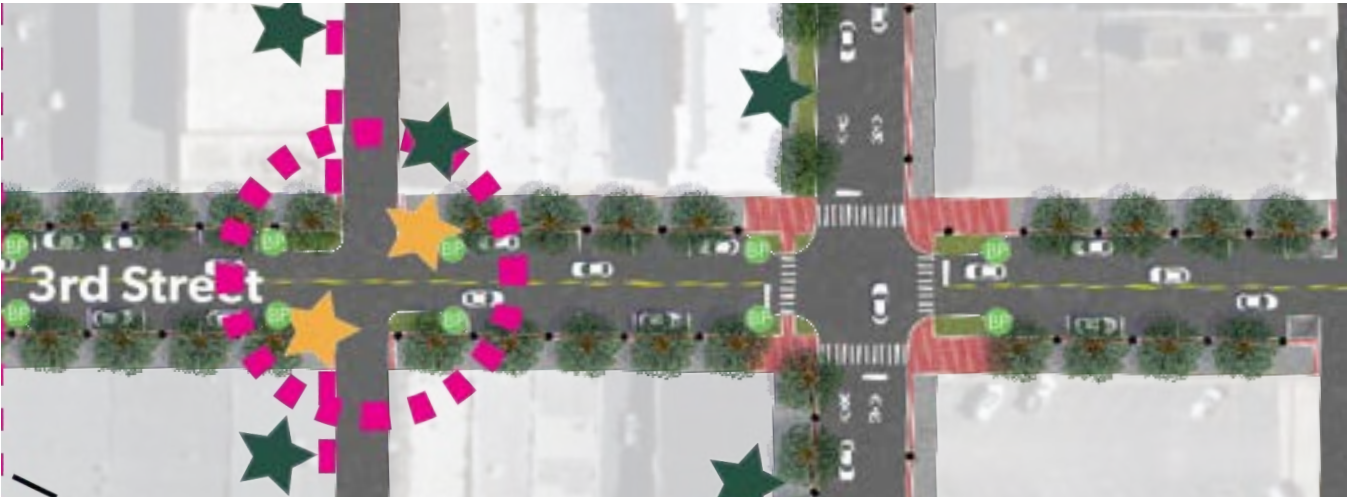
Vegetated buffers along sidewalks can filter stormwater from the roadway through a series of curb apertures.
