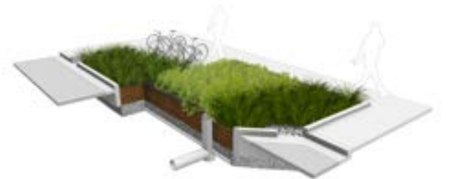
Curb apertures allow for direct stormwater flow into the bumpouts.
