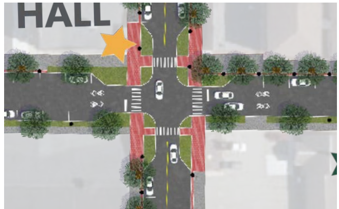
Intersection upgrades at 4th Street and Davis Avenue highlight paver sidewalk detailing and new striping.
