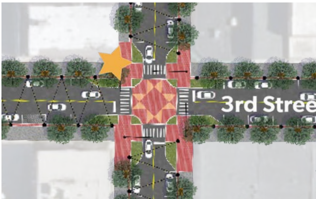
Intersection upgrades at 3rd Street and Davis Avenue include a paver intersection infill.
