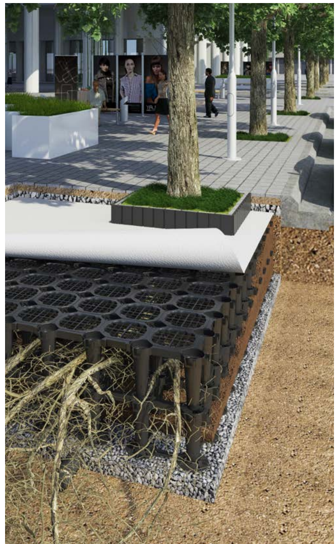
3D Visualization of a structural cell system used for street tree planting
