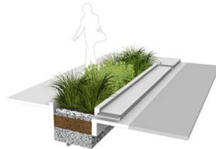
Vegetated buffers along sidewalks can filter stormwater from the roadway through a series of curb apertures.
